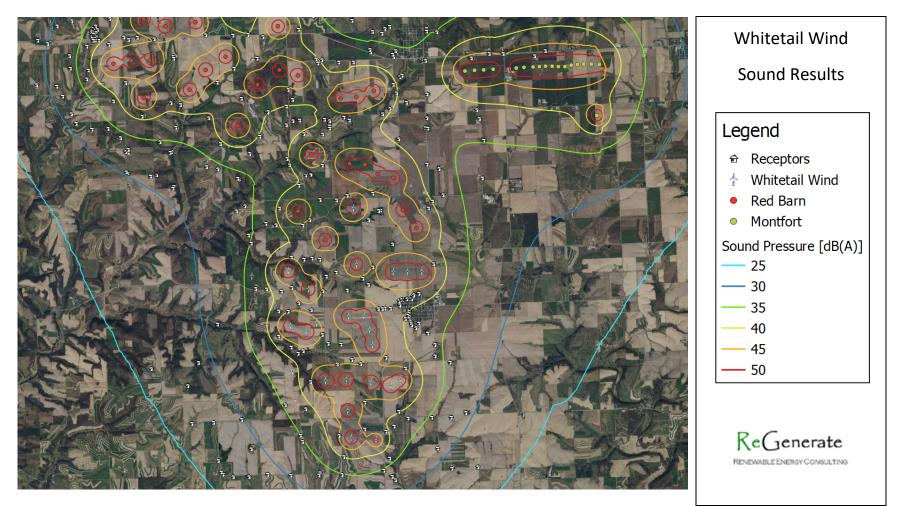
Figure 2: Sound Propagation Map of Whitetail Wind Project
